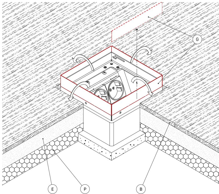
**Cross-sectional view with tabs broken out.**
